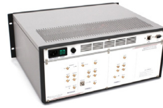
Figure 3. STX301-002R SigmaTime sub-picosecond event timer designed for the calibration of laser stations.
